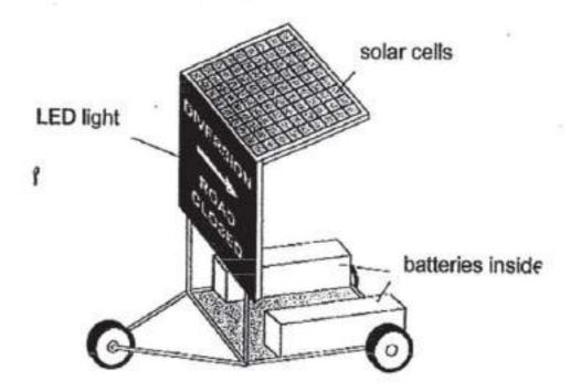
The batteries power the LED light used in the information board.
